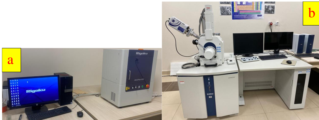
Figure 6. Microstructure test in Munzur University laboratory a) XRD, and b) SEM and EDX
