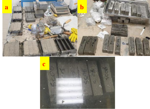
Figure 3. Sample preparation stages: a) casting, b) demolding, and c) curing
