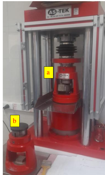
Figure 5. Compressive and flexural strength: a) flexural strength test and b) compressive strength tested on broken prisms
