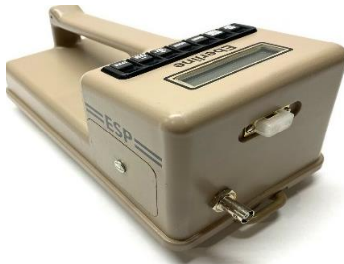
Figure 2. Eberline ESP-2 portable ratemeter coupled with an SPA-6 plastic scintillation detector for outdoor gamma-radiation measurements
