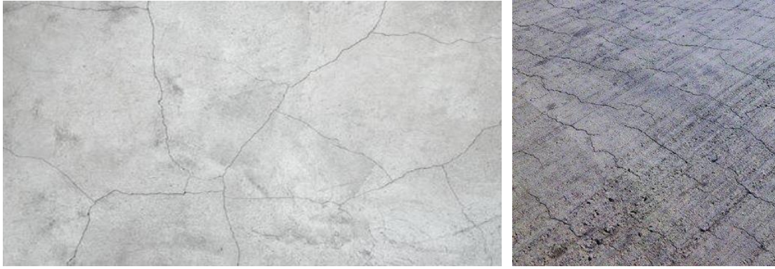
Resim 1. Plastik (erken plastik) rötire örneği [81] (Photo 1. Plastic (early plastic) shrinkage example)
