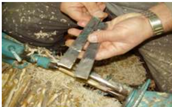
Figure 5. Stake-Knife (by Karaman 2010)
