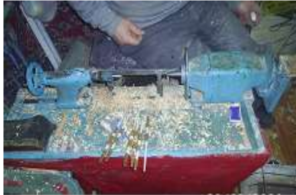
Figure 3. Lathe (by Karaman 2010)
