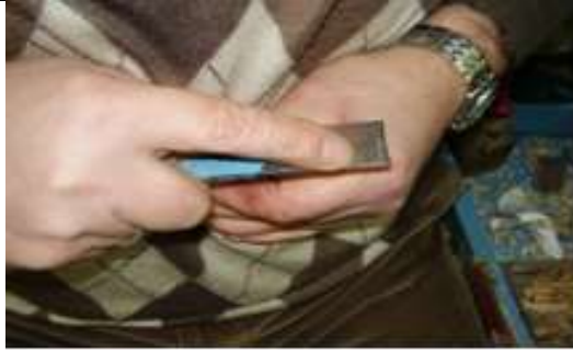
Figure 25. Carving of the Embouchure by Karaman 2010)
