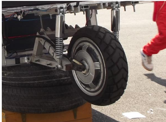
Figure 8. Anka 2014- Hub engine (2.5kW)
