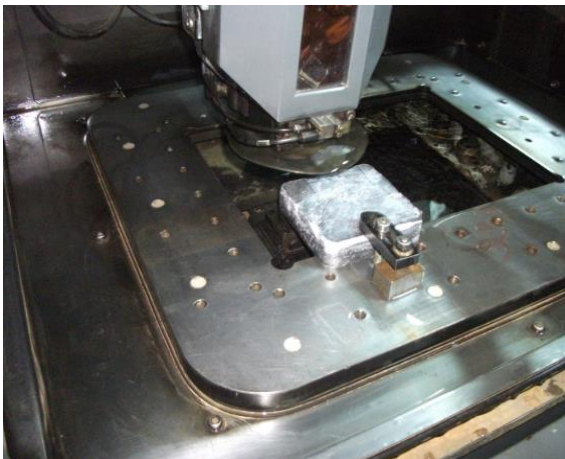
Figure 4. Preparation of samples with a wire erosion machine
