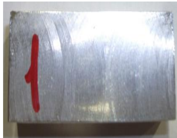
Figure 5. Samples for porosity measurement (20x20x50mm)
