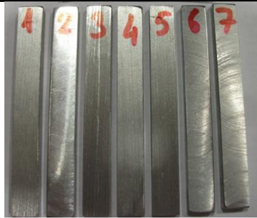
Figure 6. Samples for bending test from three points (4x10x80mm)
