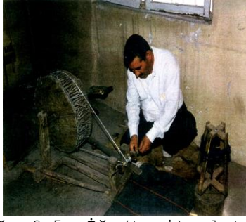
Fotoğraf 5. İğ (taşı) aleti ile iplik haline getirilen tiftik ipinin dolap ve nazuk aletleri aracılığı ile "masura"lara aktarılması, sarılması (Photo 5. Transferring and wrapping the mohair yarn, which has been made into yarn with the spindle tool, through the cupboard and the nursing equipment by means of "spools")
