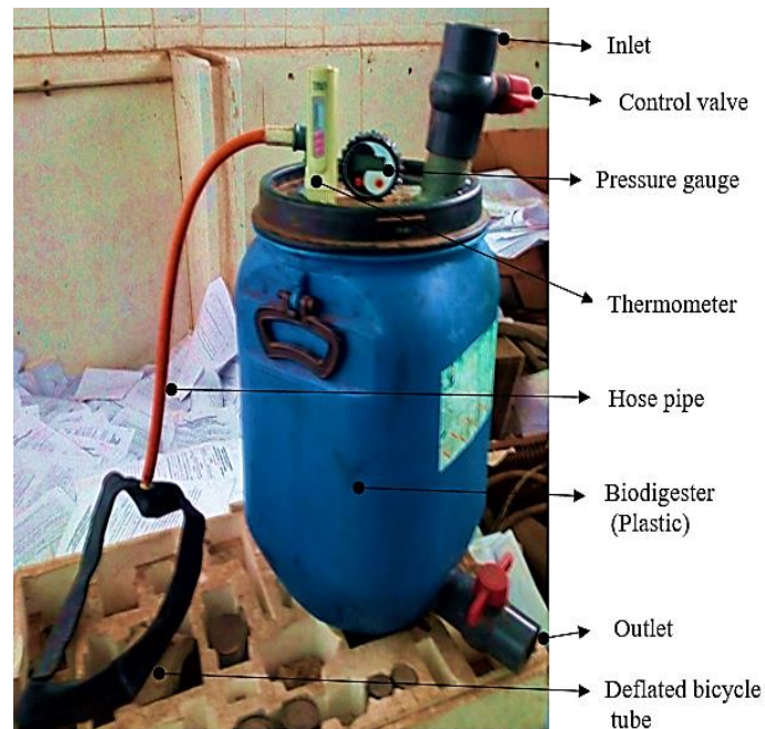
Figure 1. Experimental set-up for anaerobic digestion
