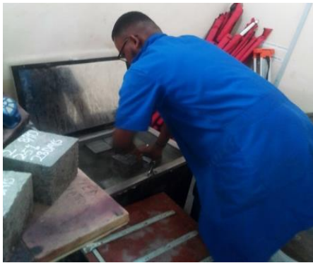
Figure 2. Curing of concrete cubes
