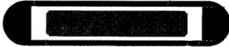
Şekil 3. Model 6711 Brakiterapi kaynağının literatürde yayınlanmış ticari şeklinin geometrisi [4] (Figure3. Geometry of commercial shape of Model 6711 seed source that was published in literature [4])
