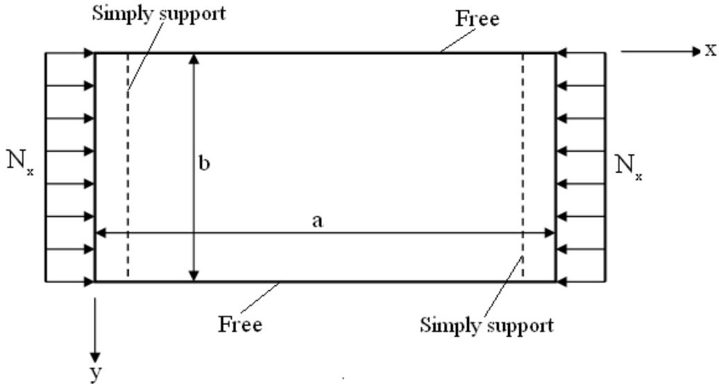
Figure 2. Geometry, loading and boundary conditions of the plate
