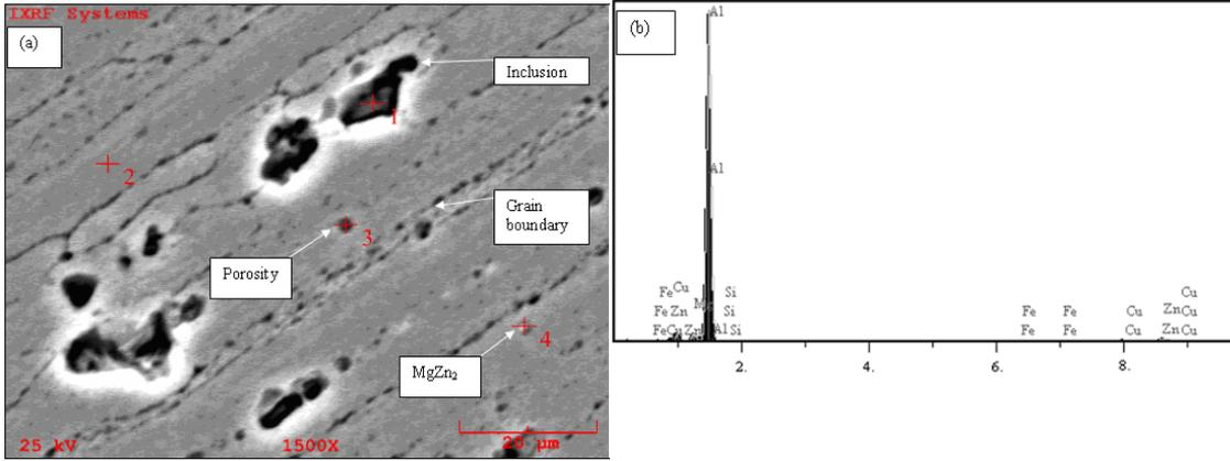
Figure 4a. SEM micrograph of the 7075 Al-alloy aged at 130°C for 48 h
