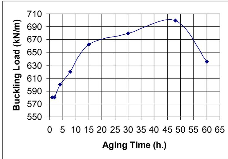
Figure 3. Buckling test results of the aged 7075 Al-alloy rectangular plate
