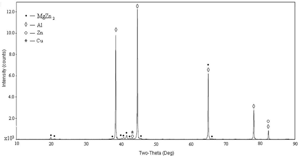
Figure 5. XRD pattern of 7075 Al alloy aged at 130°C for 48 h
