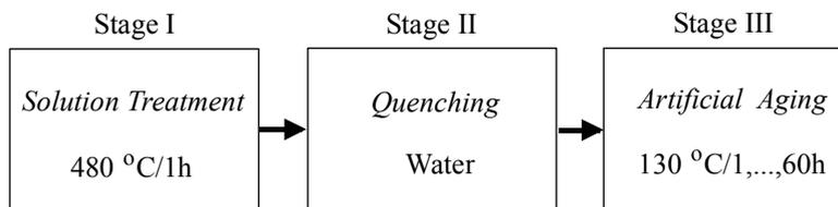
Figure 1. The heat treatment stages
