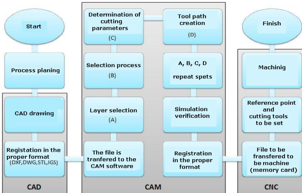
Figure 1. Integration of CAD/CAM/CNC
