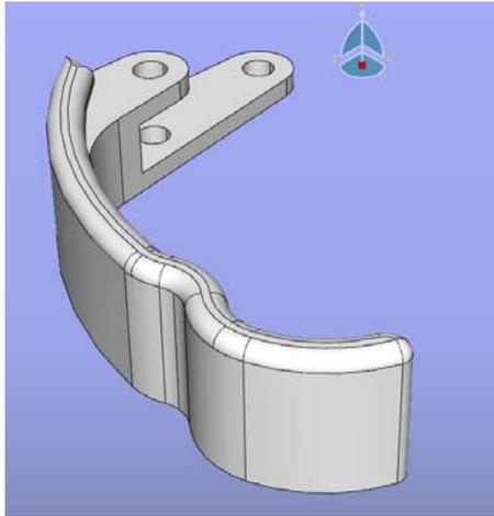
Figure 2. The Model of The Door Handle
