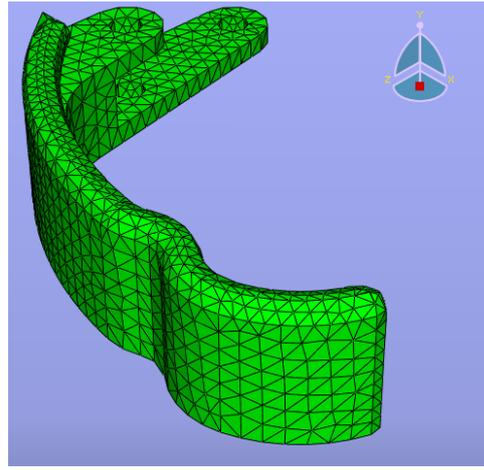
Figure 3. FEM of Mesh Door Handle
