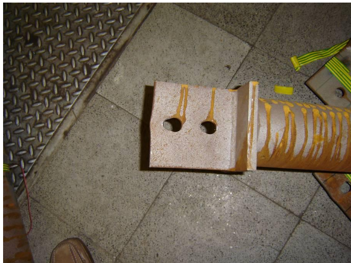
Figure 8. Cleat plate bearing (114.6x6.3 CHS tube) (Figure 8. Plaque Taquet (114.6x6.3 tube CHS))
