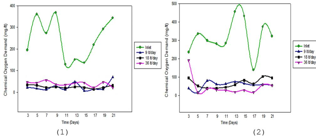
Figure 9. (1) COD removal of G soil-column (2) COD removal of K soil-column
