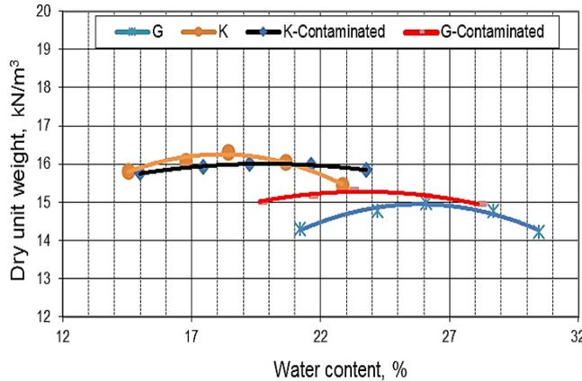
Figure 3. The effects of domestic wastewater on compaction of natural soils
