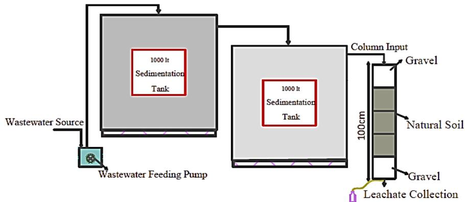
Figure 2. Schematic representation of the pilot facility (unscaled)
