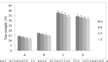
Figure 8. Tear strength in warp direction for untreated and treated fabric samples
