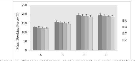
Figure 7. Tensile strength (grab method) in weft direction for untreated and treated fabric samples
