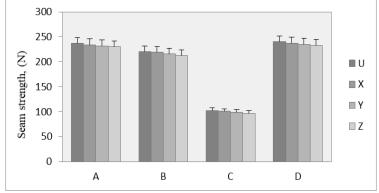
Figure 11. Seam strength in weft direction for untreated and treated fabric samples
