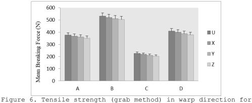
untreated and treated fabric samples
