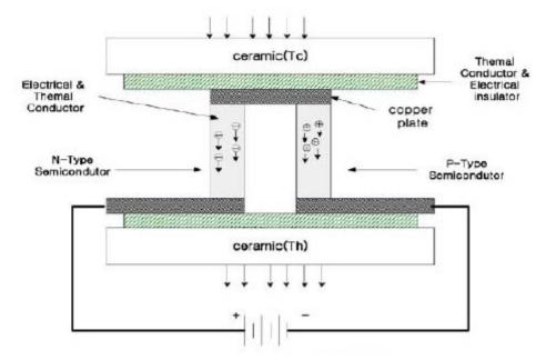
Figure 1. Principle of thermoelectric device (Sekil 1. Termoelektrik cihazın prensibi)
