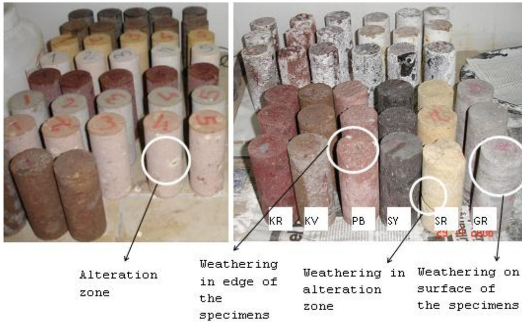
Figure 2. Visual appearance of specimens before and after salt test
