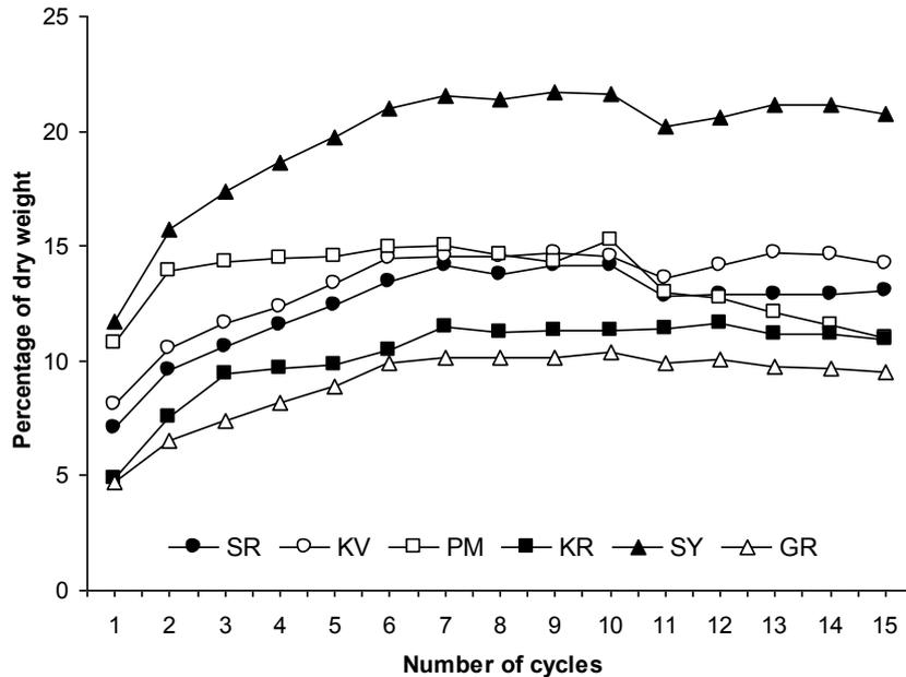
Figure 3. The percentage weight change of the tuff depends on the number of cycle[After 5]
