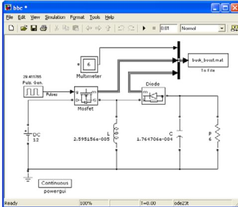
Figure 3. Simulink circuitry of the buck-boost converter
