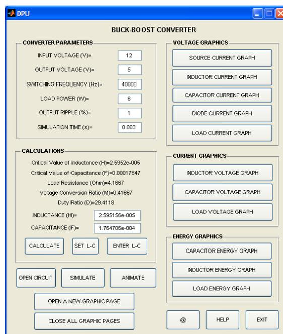
Figure 2. Individual GUI window of the buck-boost converter
