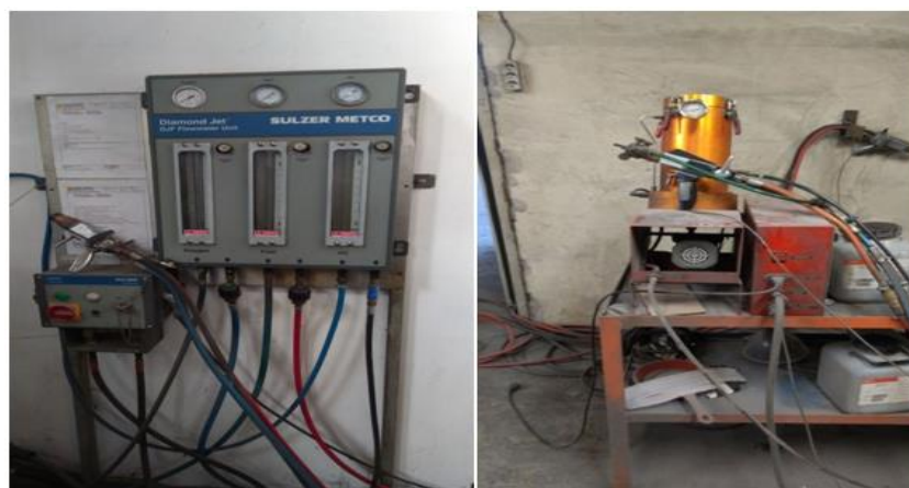
Figure 1. Plasma spray coating setup used for coating
